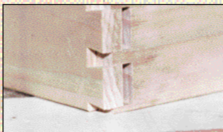
Although this joint was cut just minutes after unwrapping and assembling the unit and with no test cuts, the fit is clean and precise.
